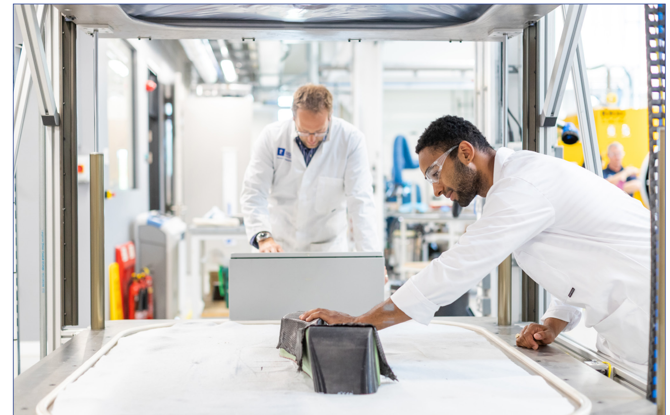
Figure 2 - Preform being removed from the Double Diaphragm Forming facility at the University of Nottingham
