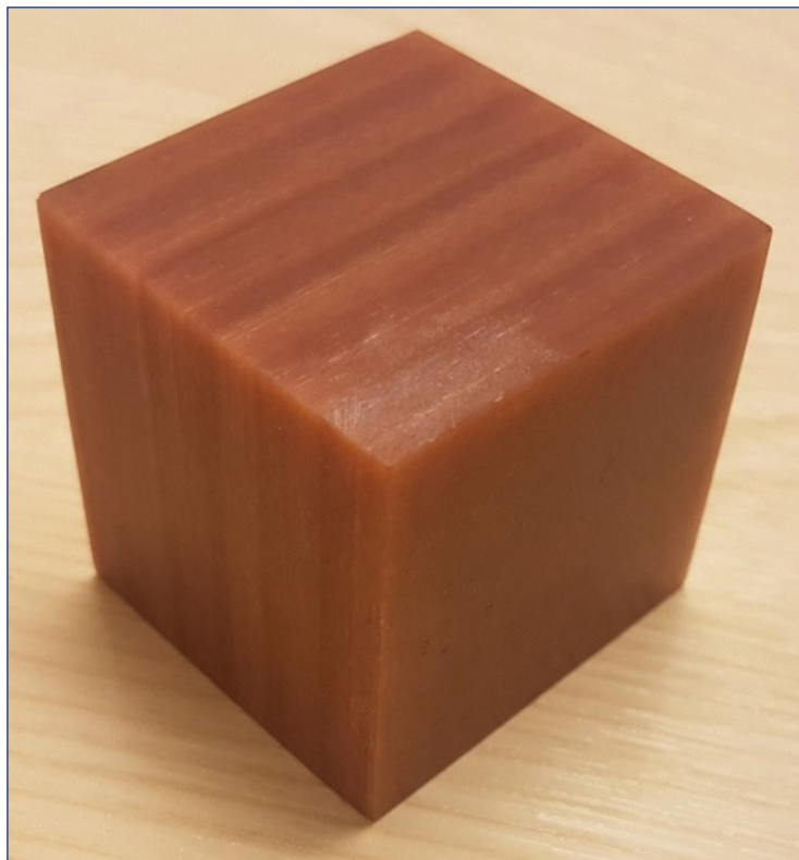
Figure 1 - 40 mm thick glass/epoxy composite successfully produced using the LbL process
