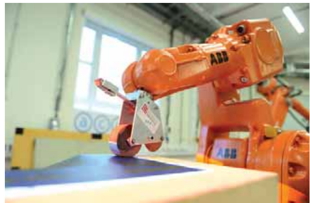
Figure 5: The automated forming of a dry fibre broadgood cloth using an ABB IRB140 6DOF robotic arm and novel end effectors to a complex geometry, also demonstrating the exploitation of low cost visualisation tools
