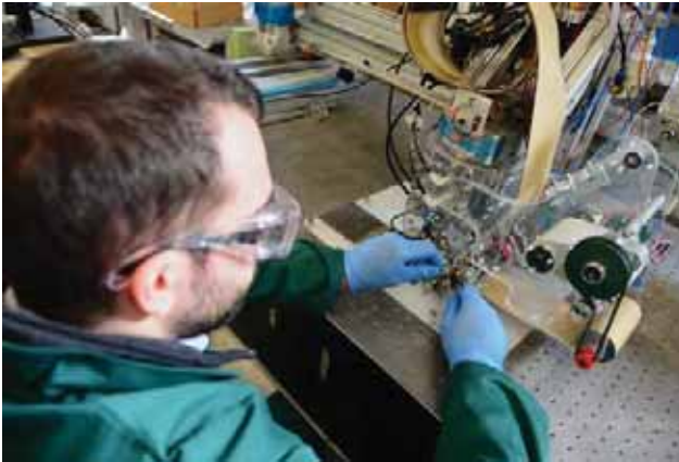
Figure 2: A researcher adjusts the wide tape continuous tow steering (CTS) machine head
