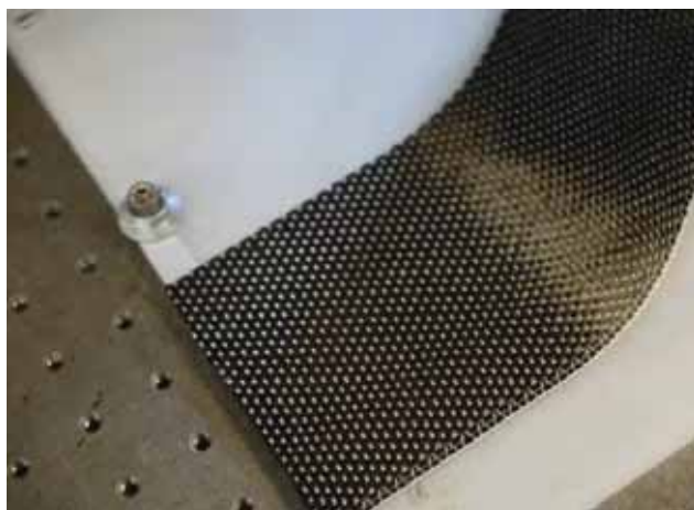
Figure 1: Automated deposition of carbon fibre tape using advanced fibre steering technology
