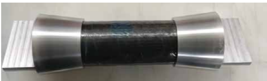
Figure 2: Thermoplastic Matrix CFC Tube with Swaged Joining to Aluminium End Fittings
