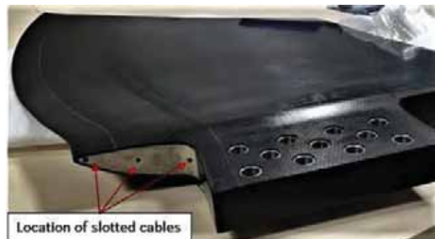
Figure 1 Location of slotted cables that provide microwave heating in composite blades
