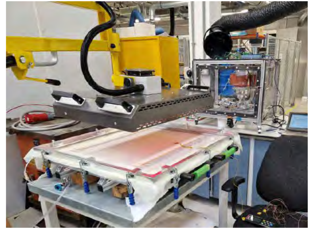
Figure 1. Caprolactam mixing and delivery system connected to double diaphragm frame, with infra-red heating.
