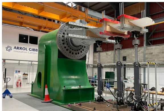
Accelerated testing of full-size tidal turbine blades at Edinburgh's FastBlade testing facility.
