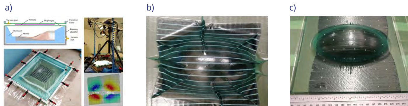
Figure 5. Double-diaphragm forming rig: a) schematic and photo, b) forming quality comparison between the continuous fibre prepreg and the HiPerDiF prepreg [formed at room temp].
