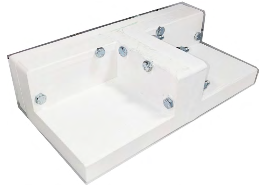
Figure 2. The demonstrator prototype: 3D printed closed mould tool
