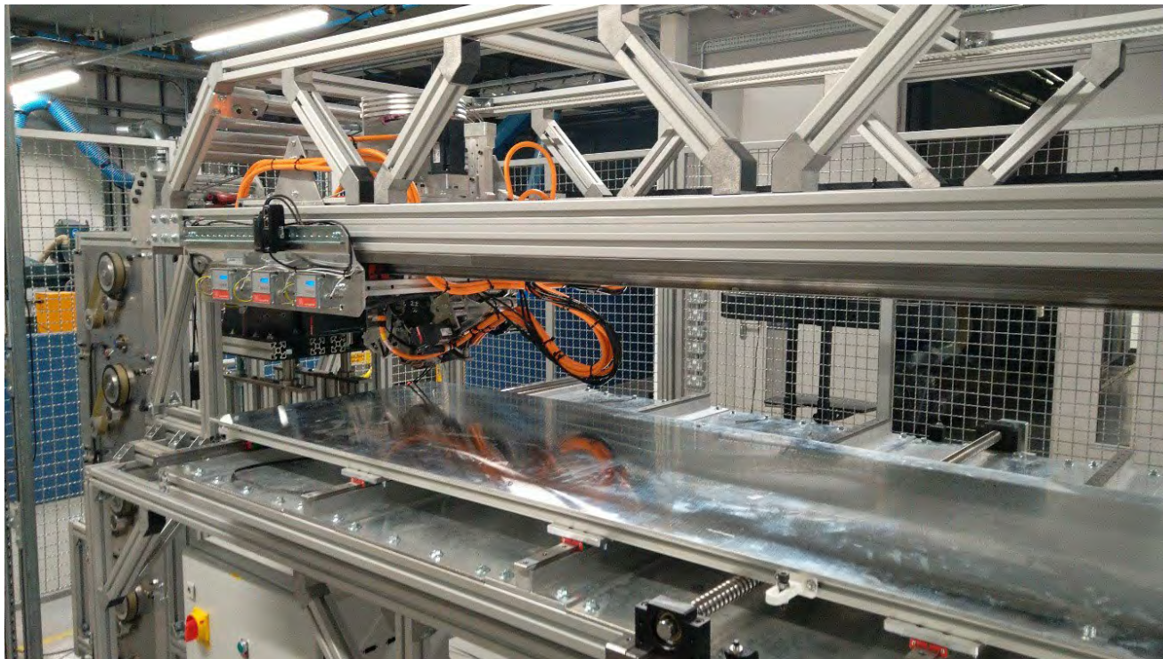
Figure 1. Automated dry fibre placement test rig incorporating digital twin under development.
