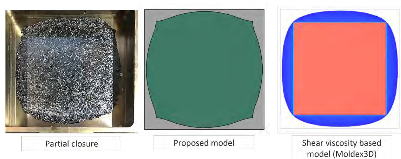
Figure 3. Comparison of filling patterns predicted by different models against the experimental partial closure
