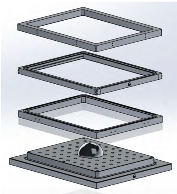
Figure 1. Small scale forming frame with vacuum base and hemisphere former.
