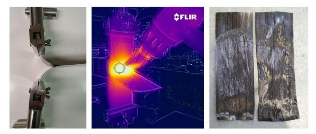
Large scale peeling of consolidated composite plies was achieved using heat and a small load. The peeled plies showed some surface disturbance but could be reprocessed into components with comparable properties to virgin plies.
