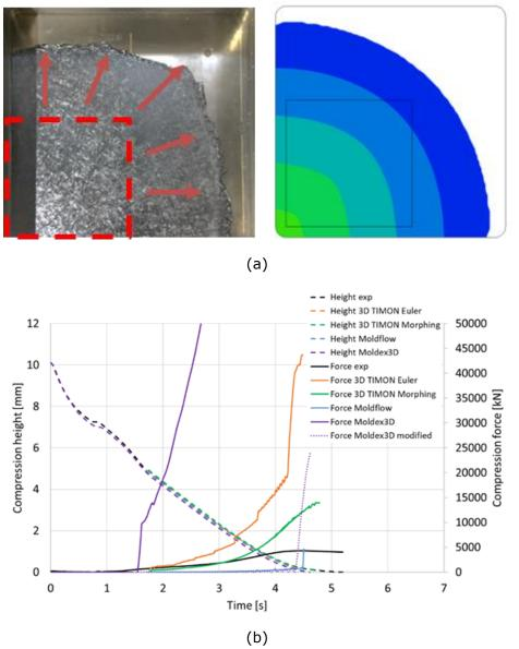
Figure 1: Case study for SMC compression moulding for a flat plaque geometry. (a) comparison of filling patterns between experiment and simulation using Moldex3D. (b) Comparison of compression forces predicted by various commercial process simulation software against the experimental data.
