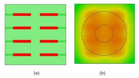
Figure 5: Optimised heating plan (a) cartridge heater layout (b) effective temperature distribution.
