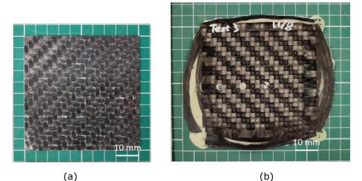
Figure 8: Comparison of prepreg compaction sample (a) before test and (b) after test.
