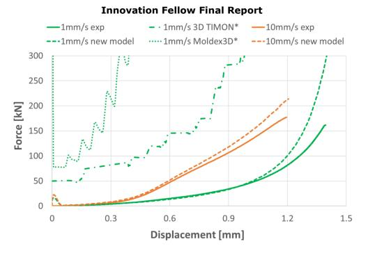
*Figure 14: Comparison of force-displacement curves from the squeeze flow tests between the proposed new constitutive model, selected commercial software and the experimental data.*
