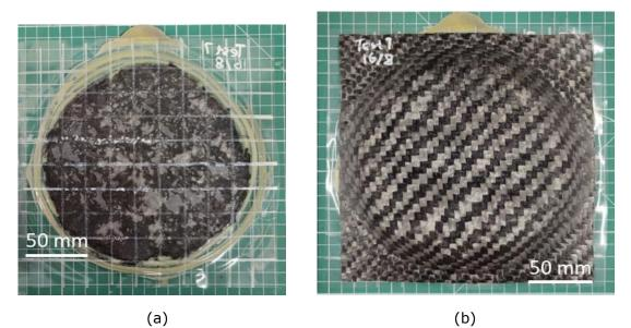
*Figure 12: Hybrid sample after compaction test (a) SMC side showing the grid lines on the film and (b) prepreg side.*
