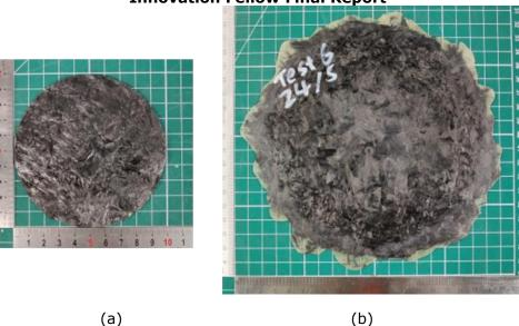
Figure 6: Comparison of an SMC squeeze flow sample (VE based, 25mm fibre length, 37%vf) (a) before test and (b) after test. The test was performed at 1mm/s closing speed and 100°C.
