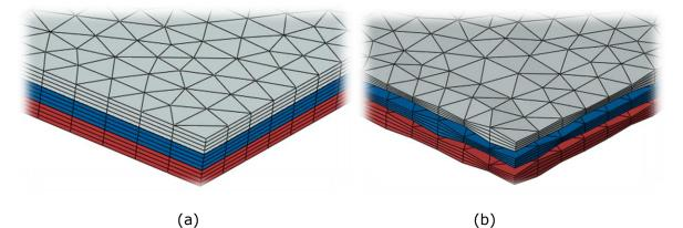
*Figure 15: Initial charge modelled using (a) regular thickness approach and (b) irregular thickness approach*
