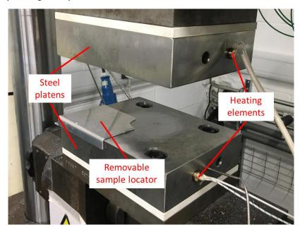
Figure 2: The old compression testing rig.
