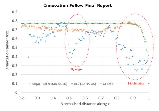
Figure 21: Comparison of fibre orientation tensor Axx distributions along the sample length between the Folgar Tucker model, the DFS model and the  $\mu$ CT data.
