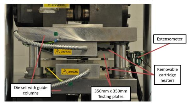
Figure 4: The new compression testing rig delivered through the project.
