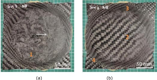
*Figure 11: Hybrid sample after compaction test (a) SMC side, (b) prepreg side. The numbers indicate important deformation mechanisms in a hybrid moulding process: 1. SMC squeeze flow; 2. Prepreg in-plane tension and out-of-plane compaction (tow spreading); 3. Prepreg in-plane compaction (tow locking) and 4, Prepreg in-plane shear (misalignment).*
