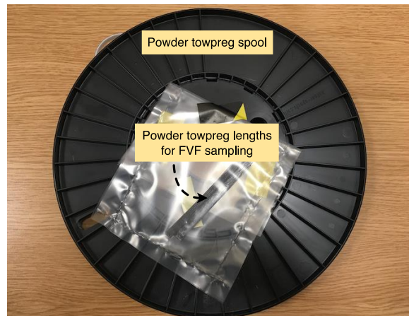
Figure 1: Powder towpreg spools produced using the tapeline
