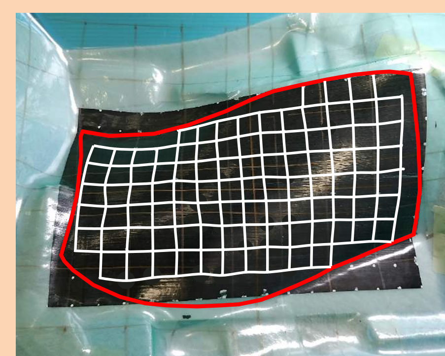
Figure 2. experimental results (left) of forming using UD prepreg with marked grids and model prediction (right) for the re-forming of prepreg tailored fibre path
