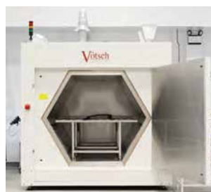
Figure 2: A mini-flow microwave reactor is used to examine the early stage microwave chemistry and curing
