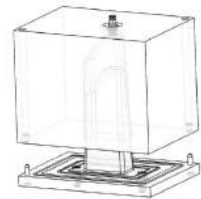
Figure 1-22 - 3D model of mold for box manufacturing
